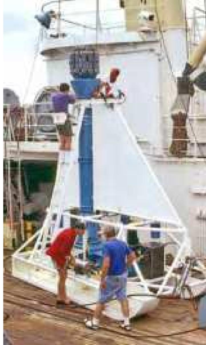
Figure 2.6: The Deep-Sea Sediment Resuspension System (DSSRS) being prepared for the BIE-II experiments. (Credit: IOM)
