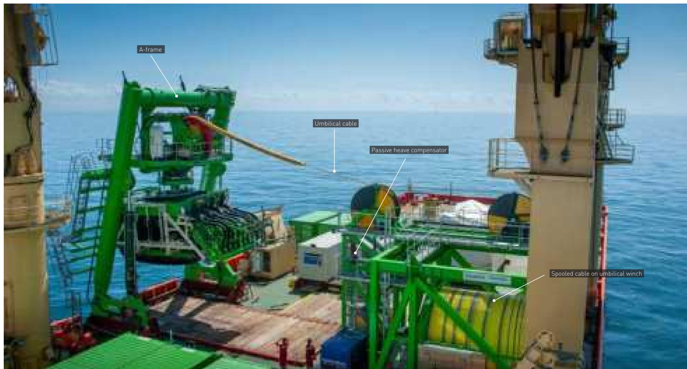
Figure 3.6: The redesigned Patania II LARS, including a passive heave compensator, being assessed during the *GSRNOD19bis* campaign in the Atlantic.
