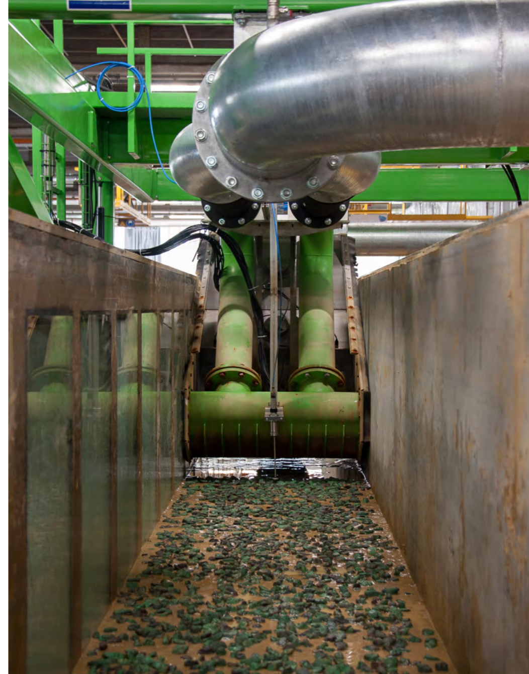
Figure 3.4: The nodule collector head testing system in the tow tank facility at the Flanders Hydraulic Research Laboratory in Antwerp, Belgium. Studies to optimize nodule pick up were performed in this facility for the ProCat1 program.
