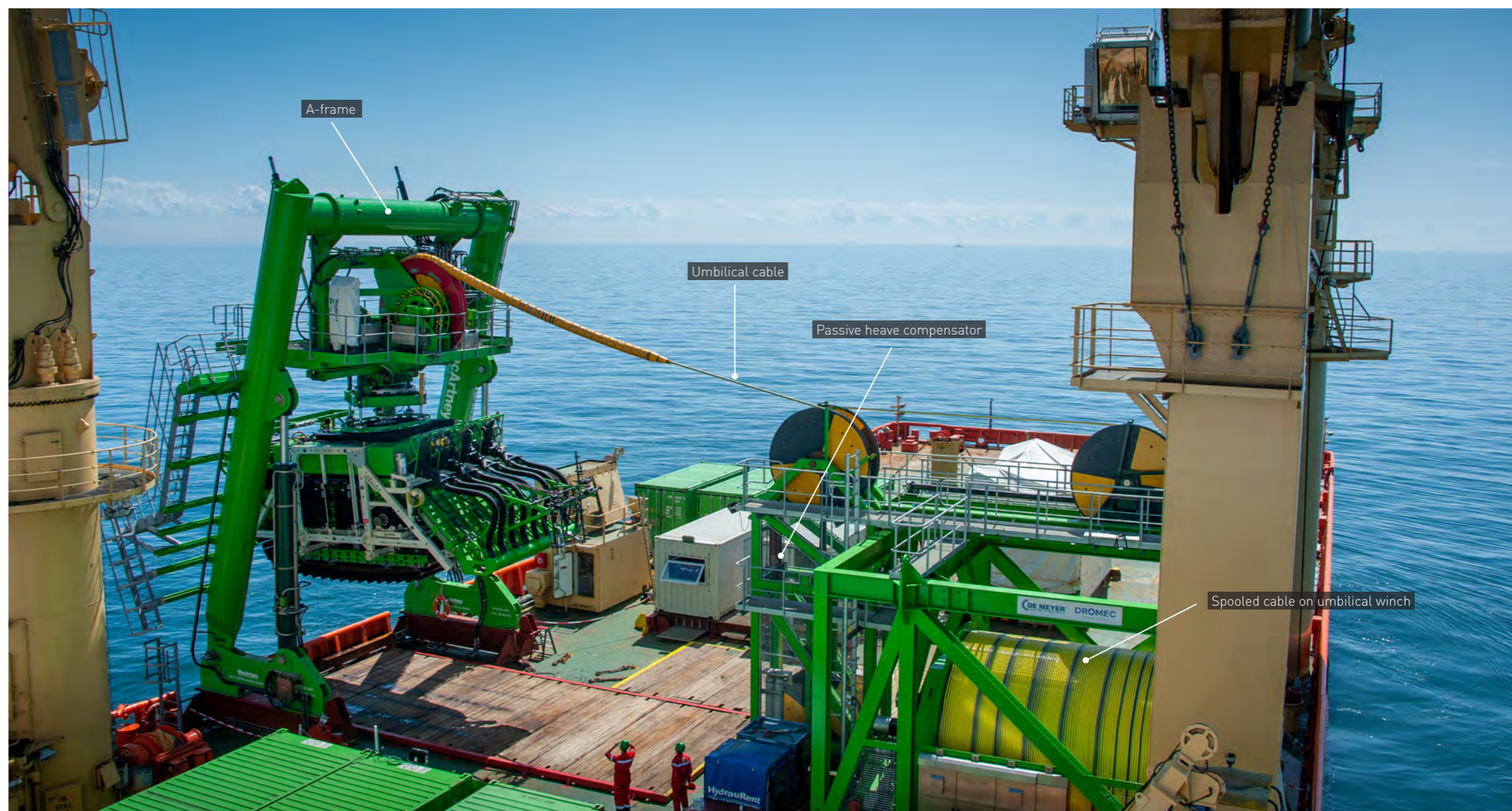
Figure 3.6: The redesigned Patania II LARS, including a passive heave compensator, being assessed during the GSRNOD19bis campaign in the Atlantic Ocean.
