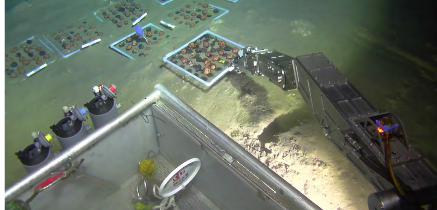
Figure 4.8: ROV manipulator arm deploying nodule frames on the seabed to conduct recolonization experiments. (Credit: MI2 & BGR)
