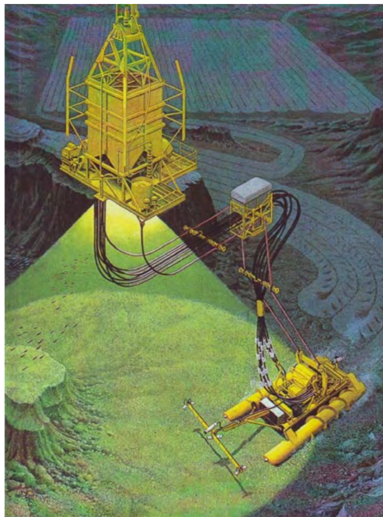
Figure 2.3: A schematic drawing of the OMCO Clementine II crawler operating on the seabed. (Credit: UKSR)
