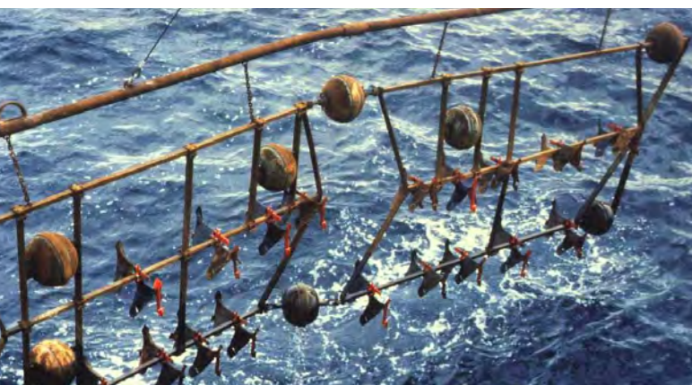
Figure 2.5: Photo of the plough harrow used for the DISCOL experiments. (Credit: G. Schriever)
