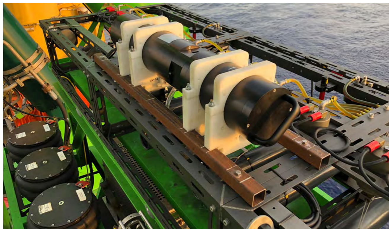
Figure 4.7: The LISST RTSSV sensor mounted at the rear, atop the Patania II.
